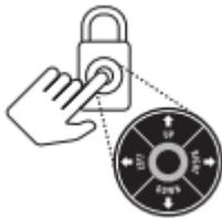
The code will be made up of directional arrows (up, down, left & right), you enter the code by waking the lock up by pushing the centre and then pushing the 4 surrounding directional buttons in the same order as your code. The lock will automatically unlock and then you can open the padlock. Your code will be active for 10 minutes prior to your booking time and expire 10 minutes after your booking time. Please ensure the lock is re-latched prior to leaving the facility.
